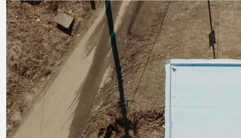
Where mod-bit roofing systems have several layers, TPO is a single-ply membrane roofing system. This innovative material is made up of polypropylene, a chemical compound known for its elasticity and durability, both of which serve it well in withstanding the Florida heat.
